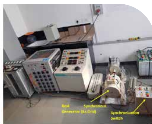
Another view of laboratory test setup for synchronizing inverter with DC motor driven SG made for islanded and grid connected mode of operations.
